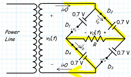
Analyzing this circuit, we find that the output voltage is:
