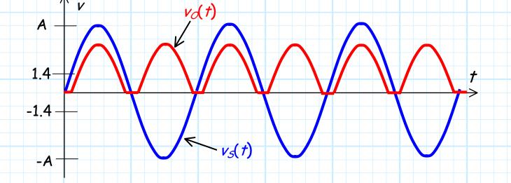
We see that the junction diode bridge rectifier output is very close to ideal. In fact, if A>>1.4 V, the DC component of this junction diode bridge rectifier is approximately:
